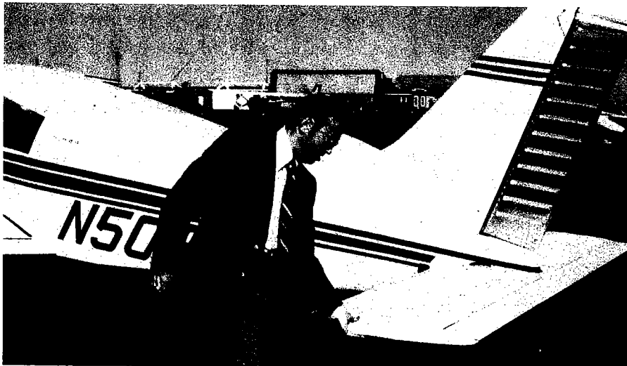
Preflight inspection requires many safety checks before the pilot even climbs into the cockpit. Above, the pilot is checking a sample of the fuel for dirt and water. For this check, a special drain is provided at low points in the fuel system. Below, the pilot is inspecting control surfaces and attachments.
